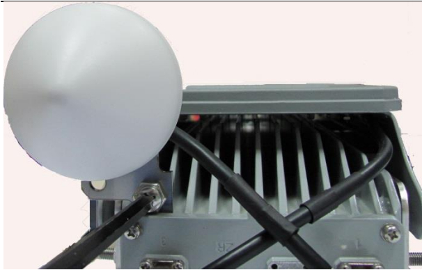
Figure 20 - Attaching the GPS antenna assembly to AirSynergy
