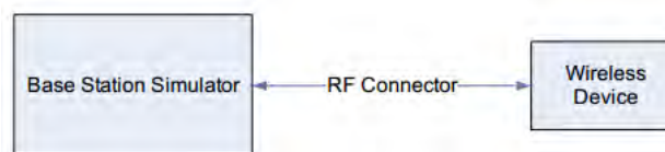
Figure 9.1 Power Measurement Setup
