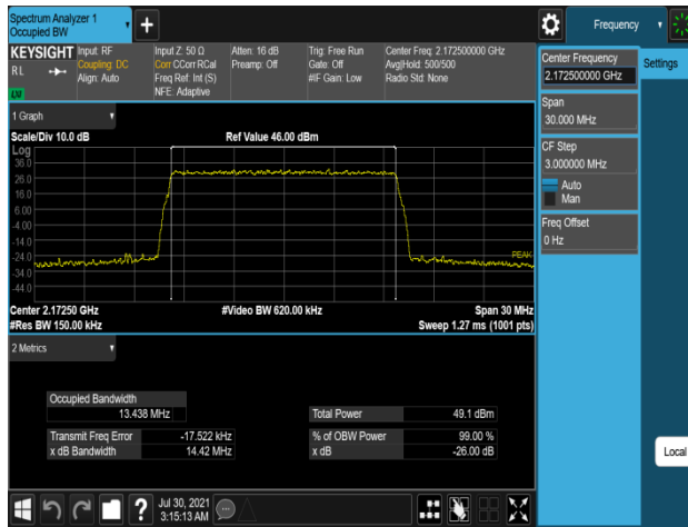
Plot 7-141. Occupied Bandwidth Plot (B66_15M_1C_QPSK - High Channel, Port 0)
