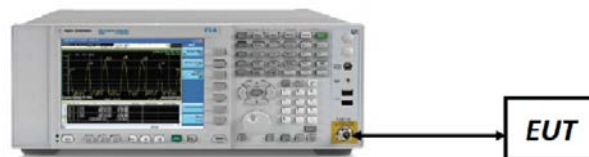
Figure 7-1. Test Instrument & Measurement Setup
