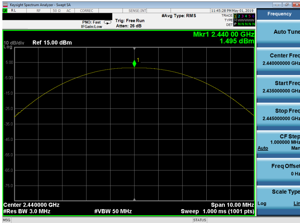
Plot 7-5. Peak Power Plot (Bluetooth (LE), 1Mbps - Ch. 19)
