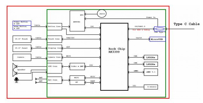
The AMPAK Technology® AP6398SV is a fully Wi-Fi and Bluetooth functionalities module with seamless roaming capabilities and advance security, also it could interact with different vendors' 802.11a/b/g/n/ac 2x2 Access Points with MIMO standard and can accomplish up to speed of 866Mbps with dual stream in 802.11ac to connect the wireless LAN. Furthermore AP6398SV included SDIO interface for Wi-Fi, UART/ PCM interface for Bluetooth.
