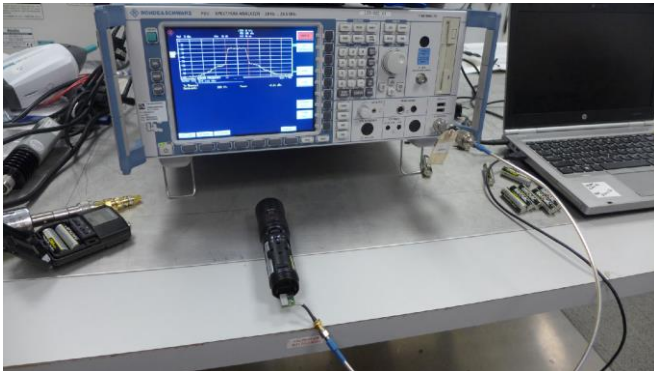
Figure 1: Test setup for Maximum Radiated Output
