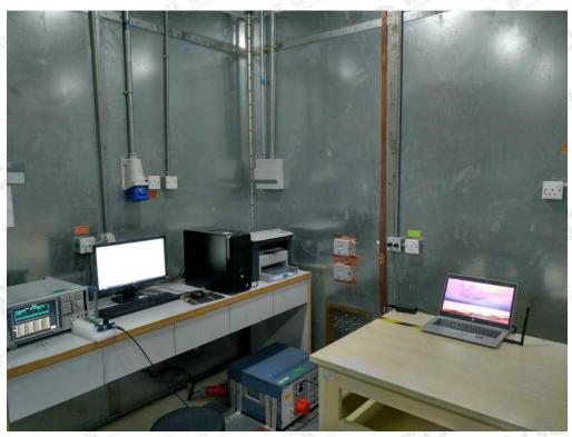
FCC RADIATED EMISSION TEST SETUP BELOW 1GHZ
