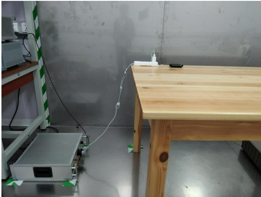
Conducted Emission at AC power line
