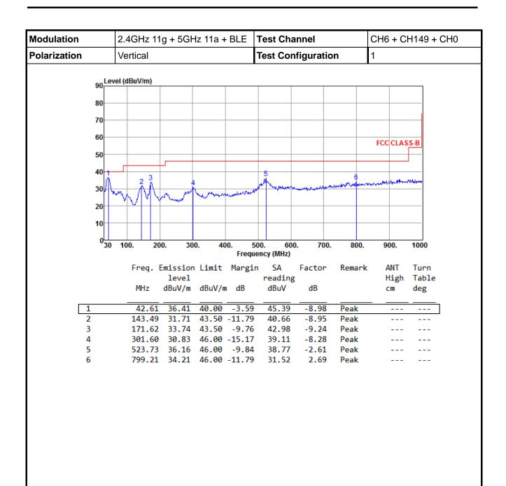
Note 1: Emission Level (dBuV/m) = SA Reading (dBuV/m) + Factor\* (dB)
