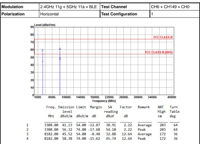
Note 1: Emission Level (dBuV/m) = SA Reading (dBuV/m) + Factor\* (dB)
