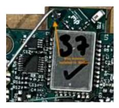
Once the module is complete it is then installed by soldering on to the main PCBA of 1 of 3 host boards. The DWE-DT1 (Host), the DWE-CT1 (Host) and or the DWE-DH1 (Host) as shown in the below photo
