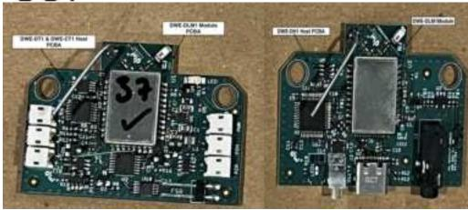
The module/host PCBAS are now ready to install into their respective host mechanicals to complete final host assembly.
