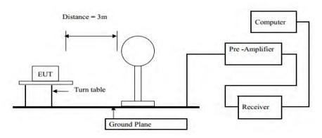
Semi-Anechoic 3m Chamber
