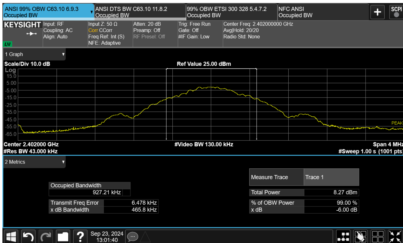
Figure TR09.3: Occupied bandwidth data for ANT at low channel (2402 MHz)
