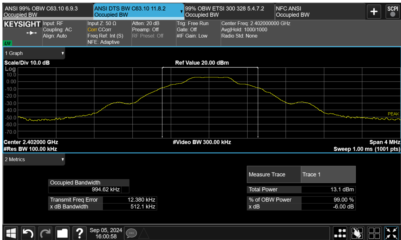
Figure TR05.2: Bandwidth data for Bluetooth BR at channel 2402 MHz
