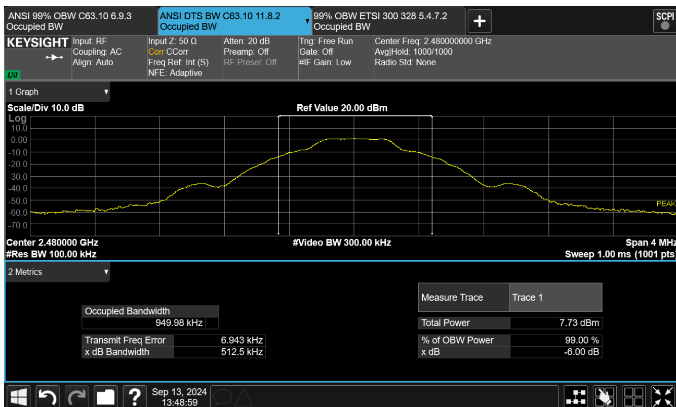
Figure TR05.7: Bandwidth data for ANT at channel 2480 MHz
