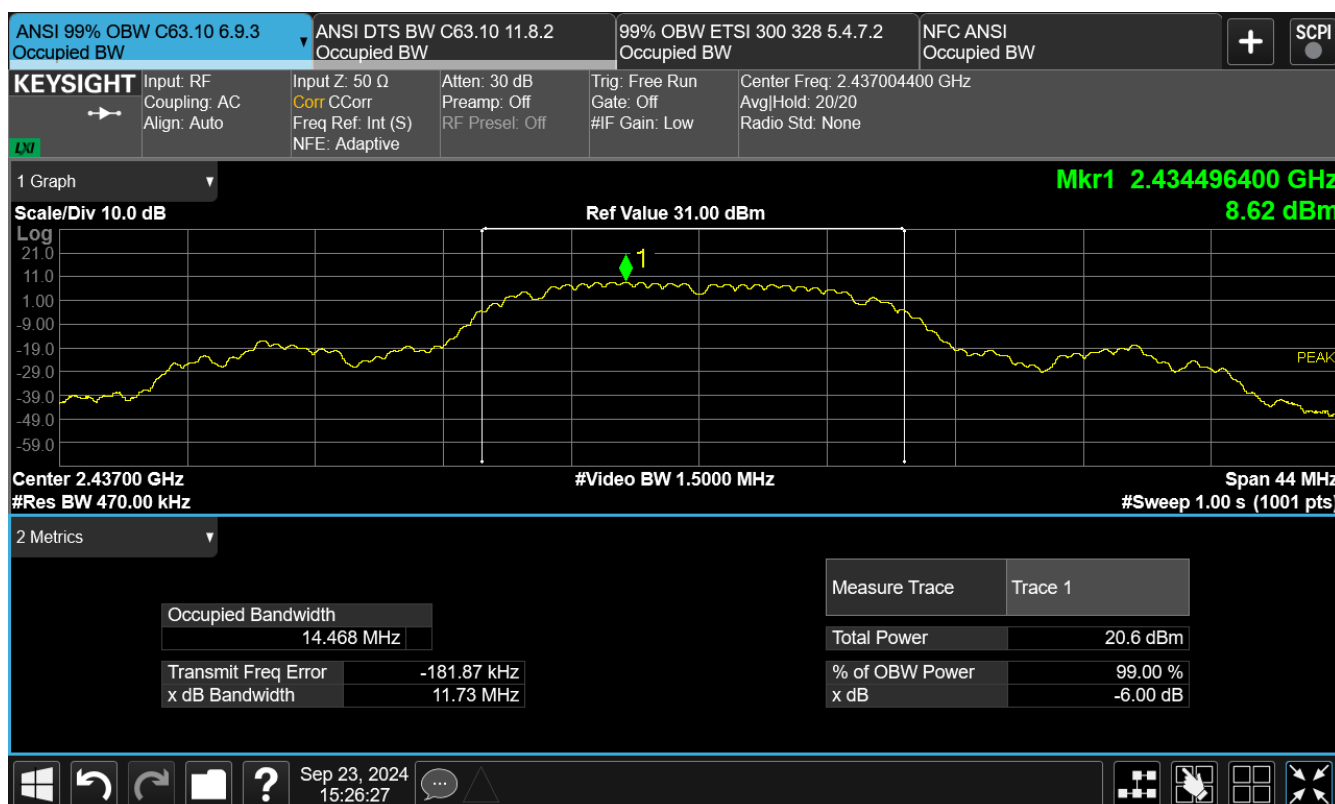
Figure TR09.4: Occupied bandwidth data for 802.11b 1 Mbps at channel 6
