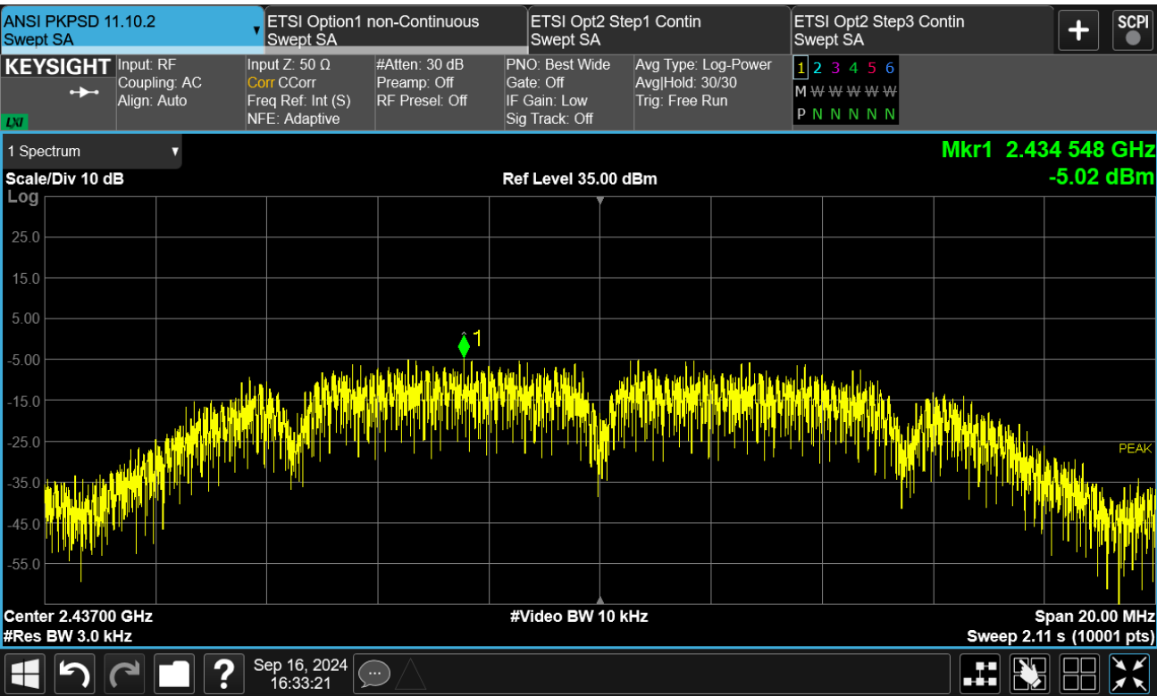
Figure TR18.5: Test data for IEEE 802.11 B2 modulation, channel 6
