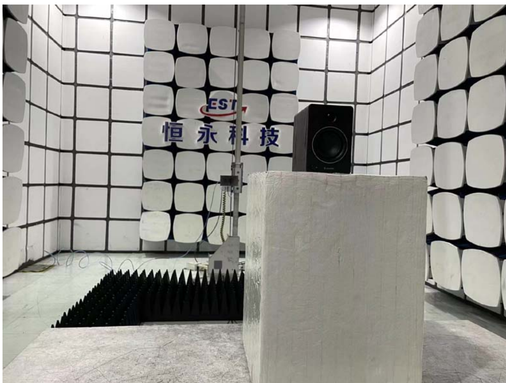
Radiated emission test: Above 1GHz
