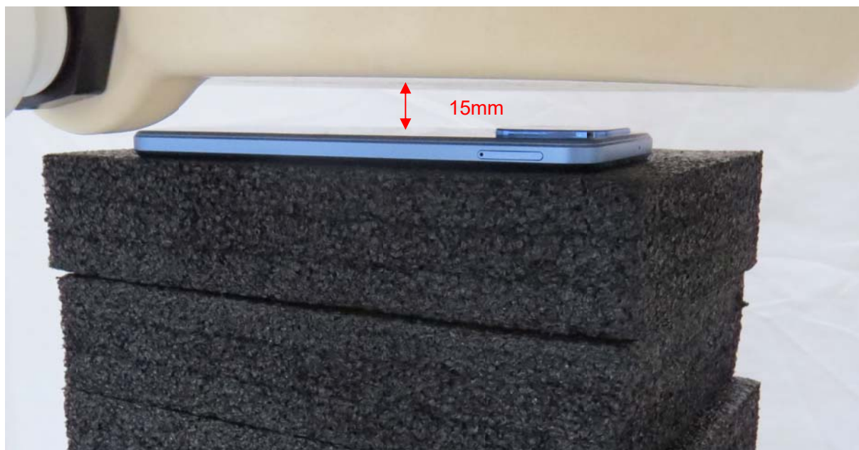
Picture 5: Back Side, the distance from handset to the bottom of the Phantom is 15mm
