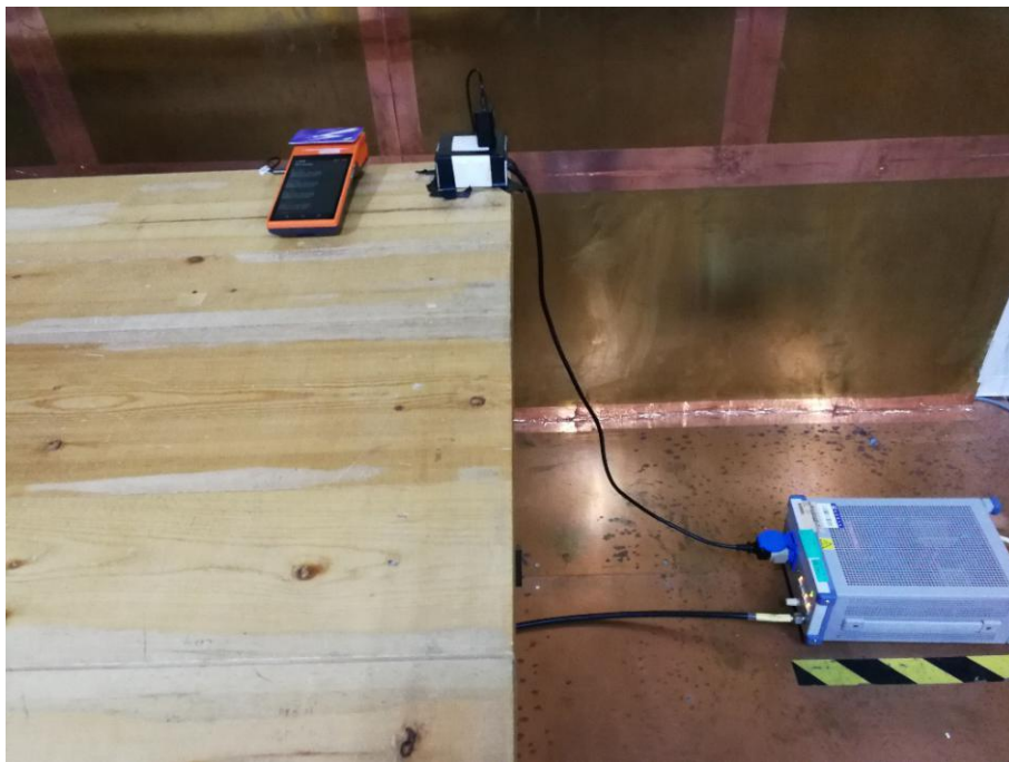
Description: Conducted Emissions Test Setup (NFC)
