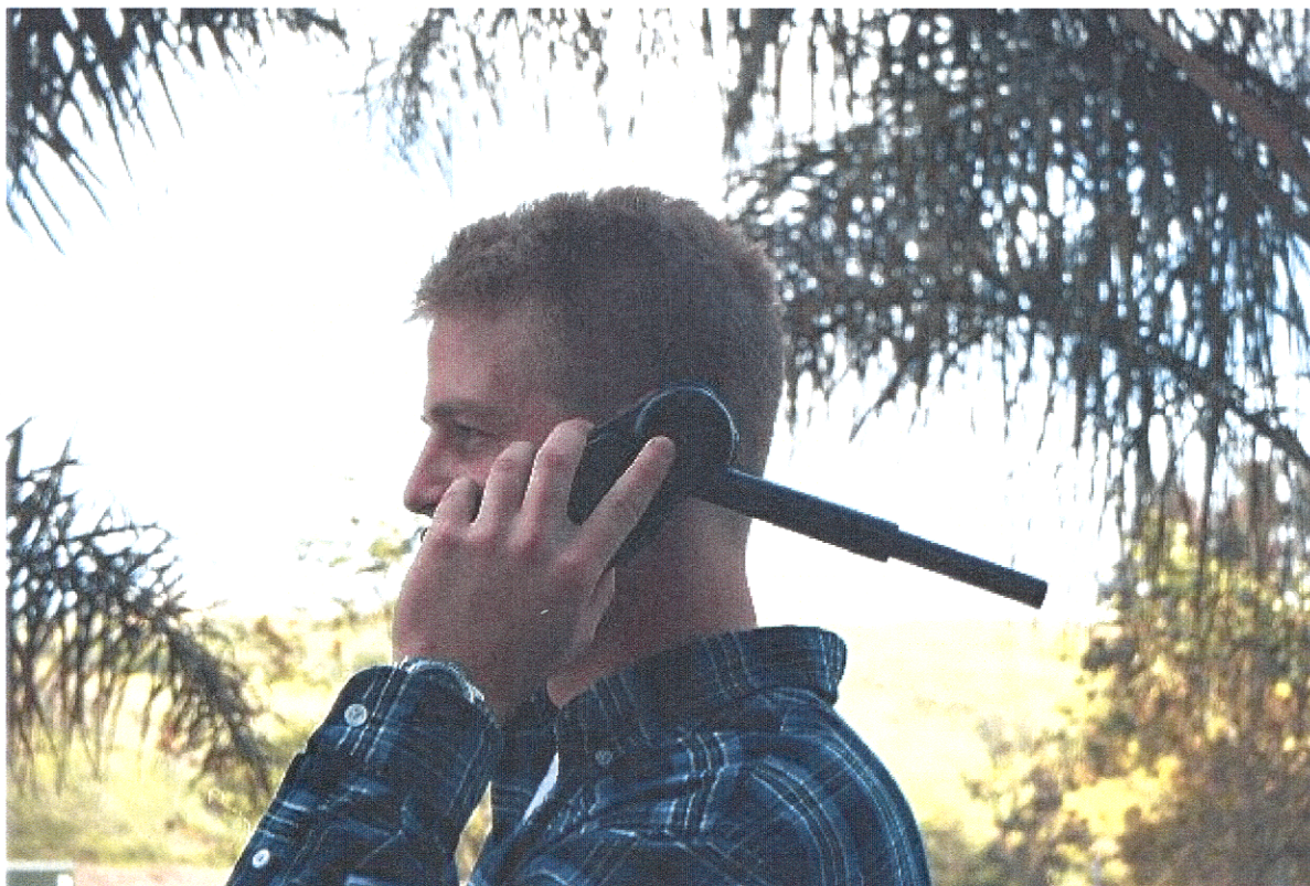
Photo 13 – GSP 1610 With Incorrect Antenna Position
