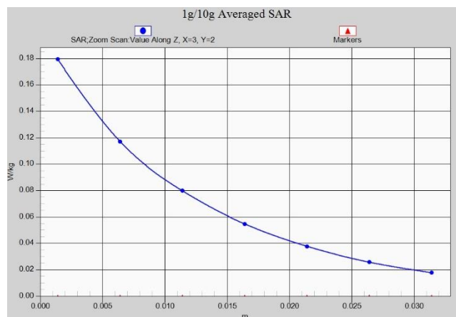
Fig. 1-3 Z-Scan at power reference point (PCS1900)
