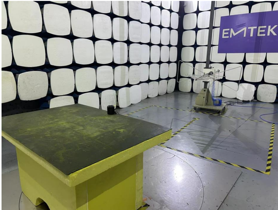
Spurious Emission Test Setup (Below 1GHz)
