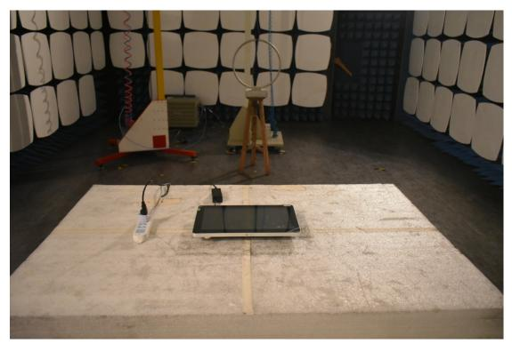
3. Radiated emission (9KHz-30MHz)
