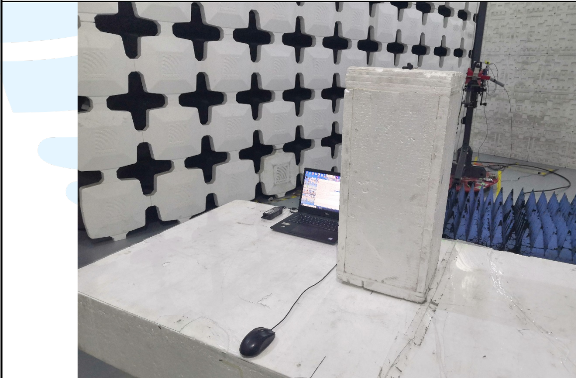
Radiated emission Test Setup (Above 1 GHz)
