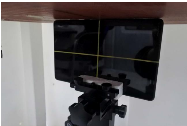
Edge 2 of EUT with Phantom 0 mm Gap
