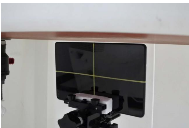
Edge 4 of EUT with Phantom 6 mm Gap
