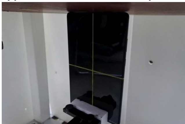
Edge 1 of EUT with Phantom 0 mm Gap
