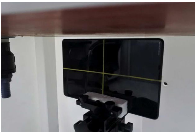
Edge 2 of EUT with Phantom 4 mm Gap
