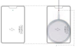
Ensure that the charging position is aligned with the wireless charger
