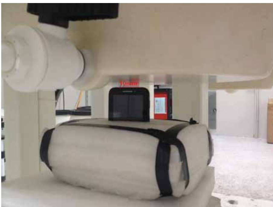
Body SAR Right Side 10mm for GSM/UMTS
