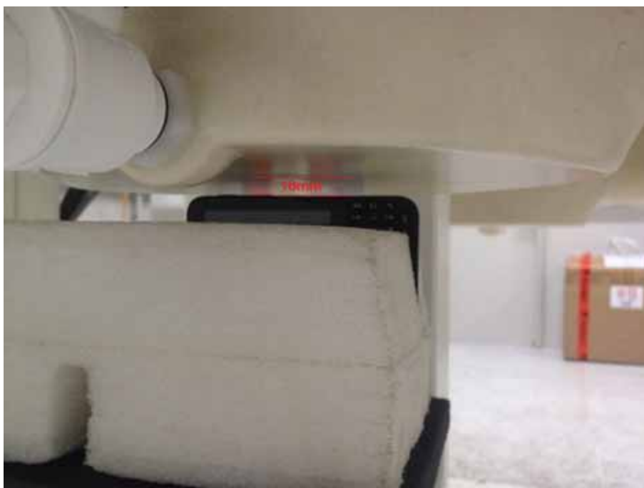
Body SAR Right Side 10mm for GSM/UMTS
