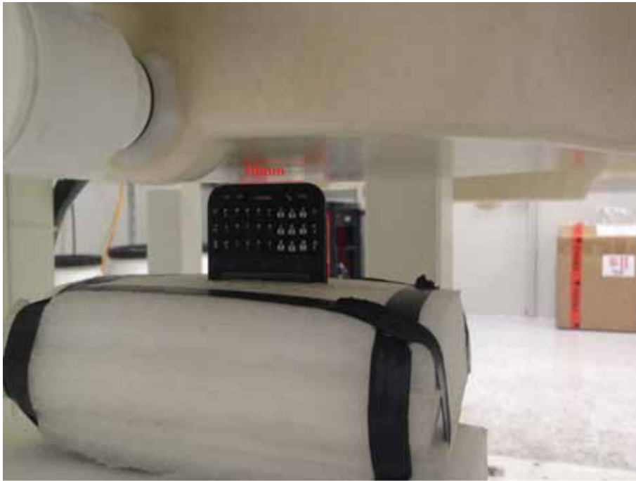
Body SAR Bottom 10mm for GSM/UMTS
