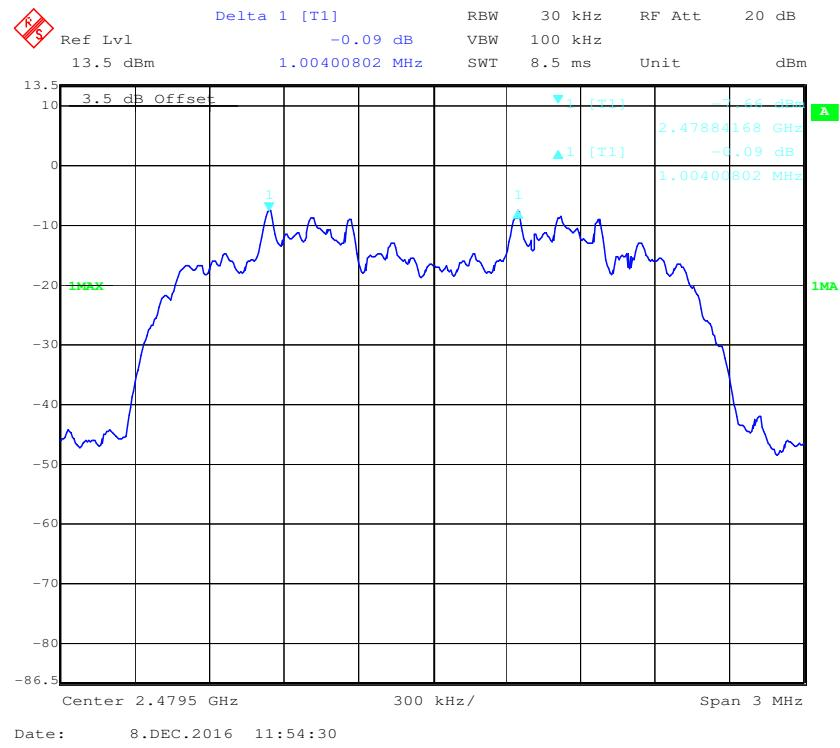
**EDR (8DPSK): Low Channel**
