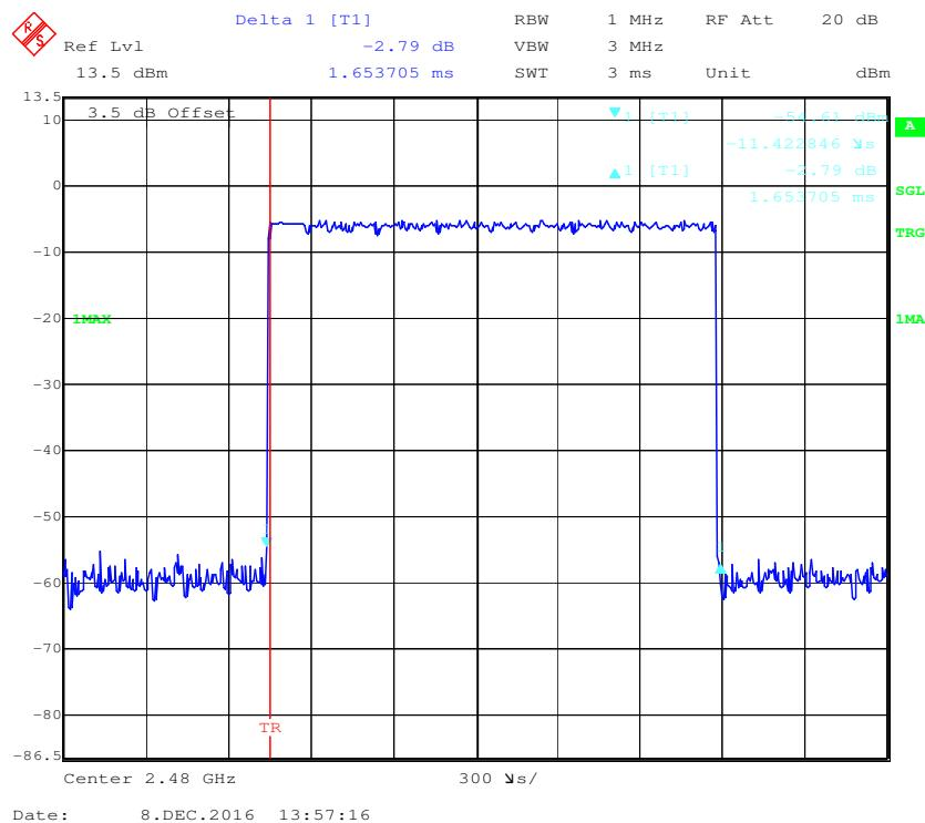
**Pulse time, Low Channel, 3DH5**
