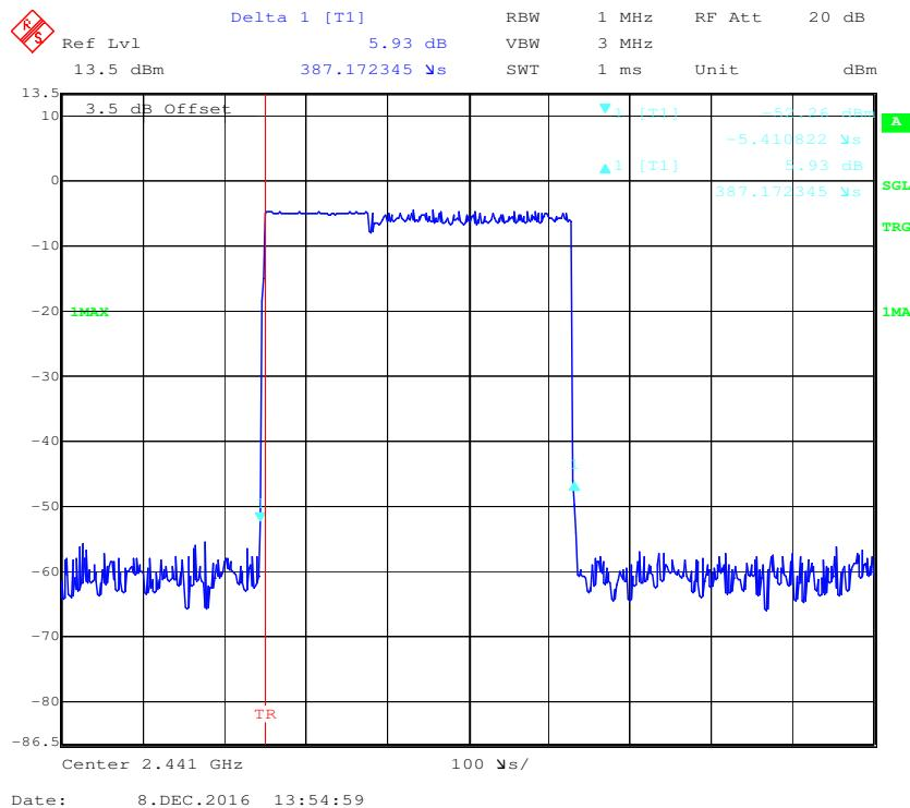
**Pulse time, High Channel, 3DH1**
