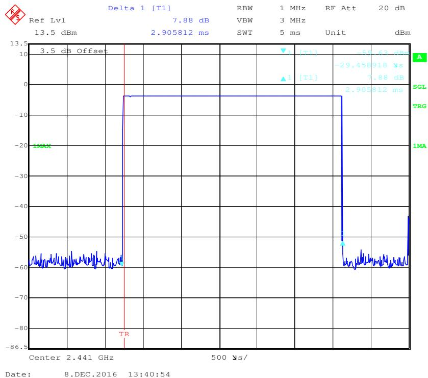
**Pulse time, High Channel, DH5**
