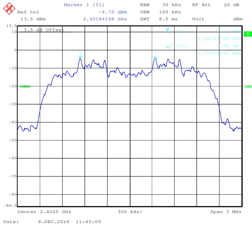
**EDR ( $\pi/4$ -DQPSK): Middle Channel**
