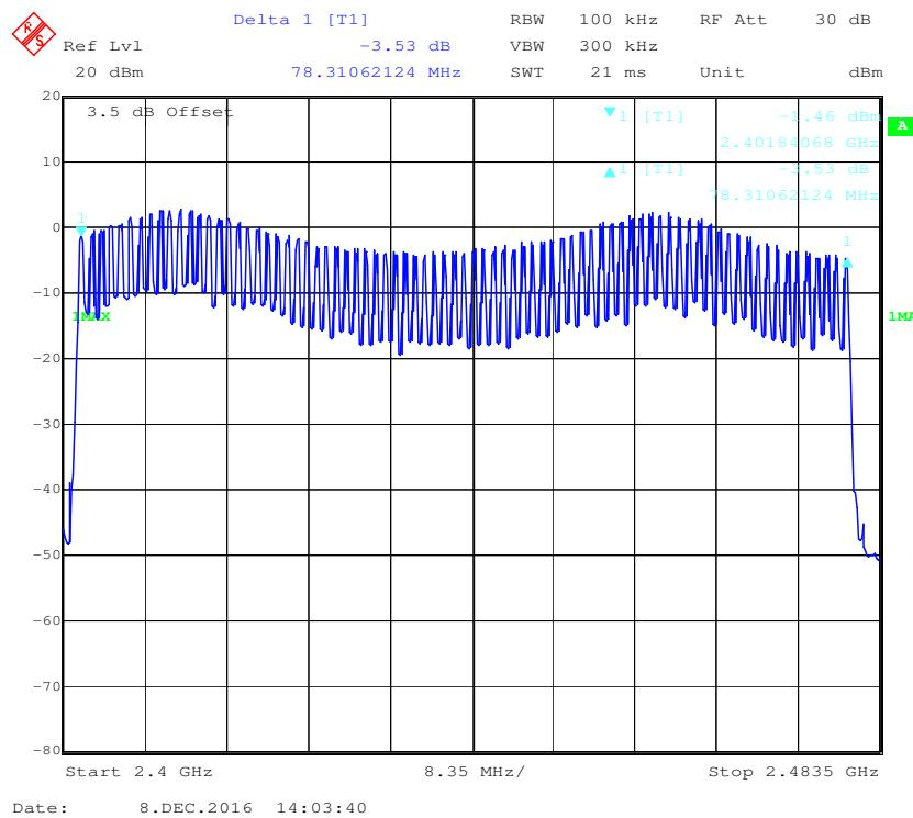
**EDR ( $\pi/4$ -DQPSK): Number of Hopping Channels**
