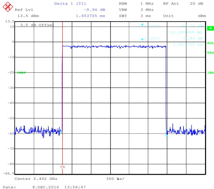
**Pulse time, Middle Channel, 3DH3**
