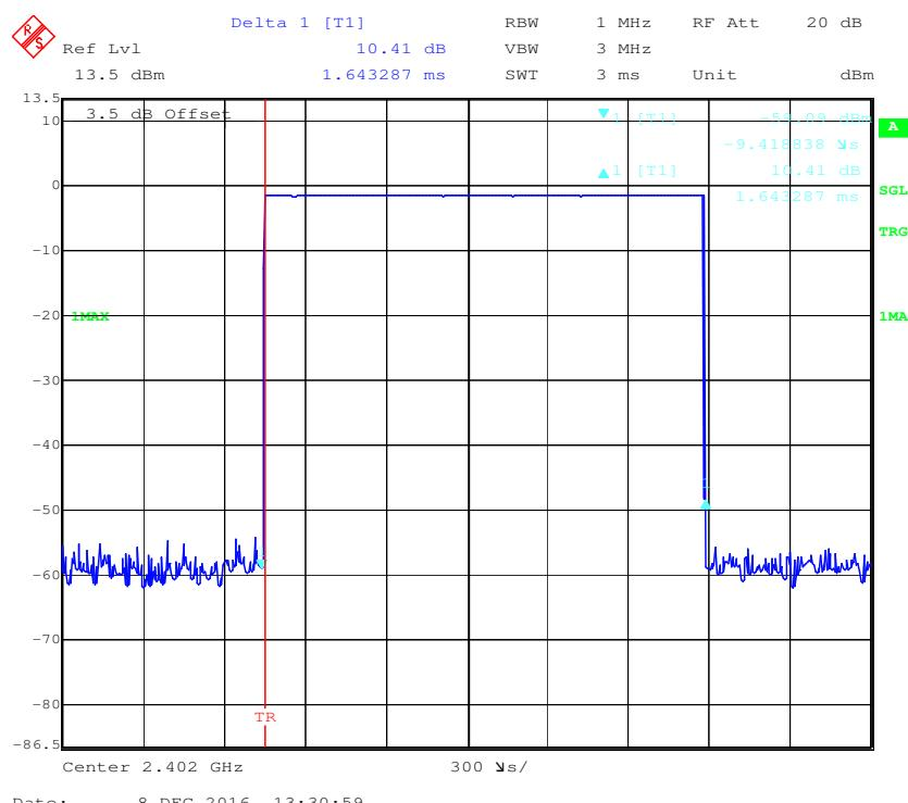
**Pulse time, Middle Channel, DH3**
