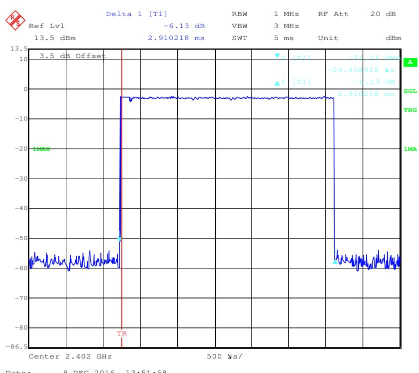
**Pulse time, Middle Channel, 2DH5**
