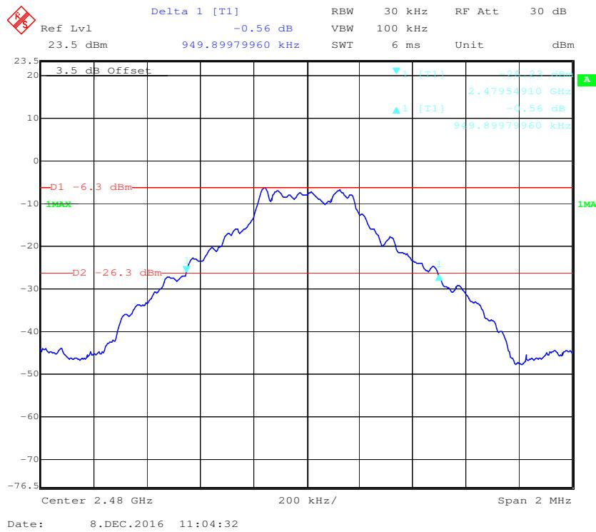
**EDR ( $\pi/4$ -DQPSK): Low Channel**
