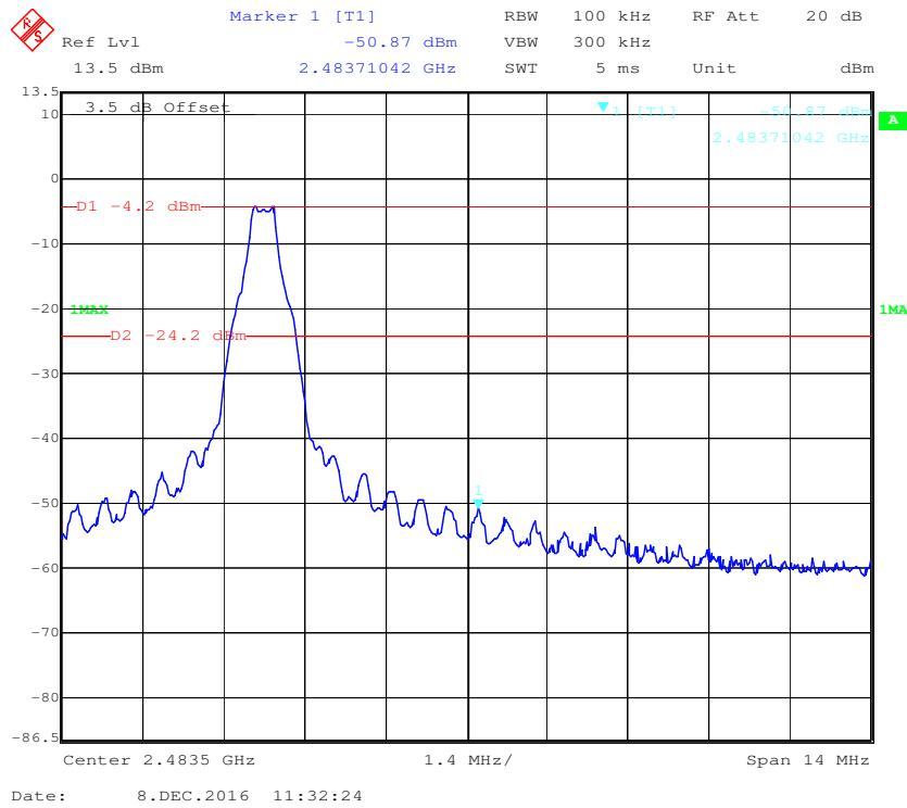
**EDR ( $\pi/4$ -DQPSK): Band Edge-Left Side**
