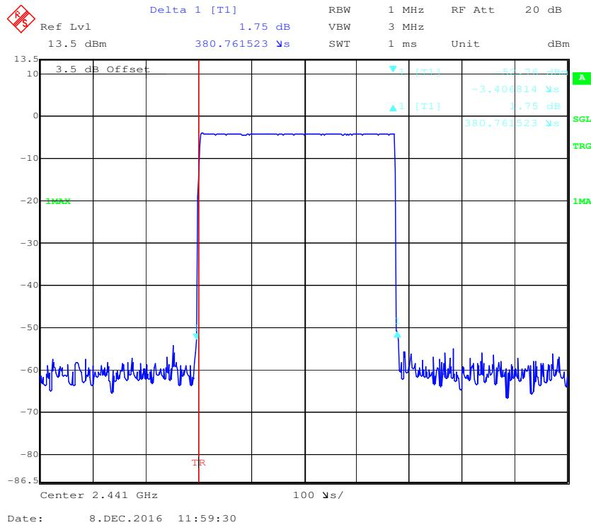
**Pulse time, High Channel, DH1**
