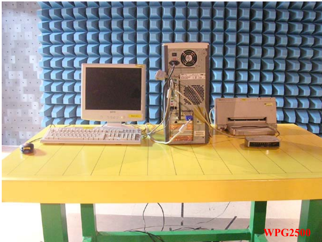
Photo 1: Radiated Emission Test Set-up
