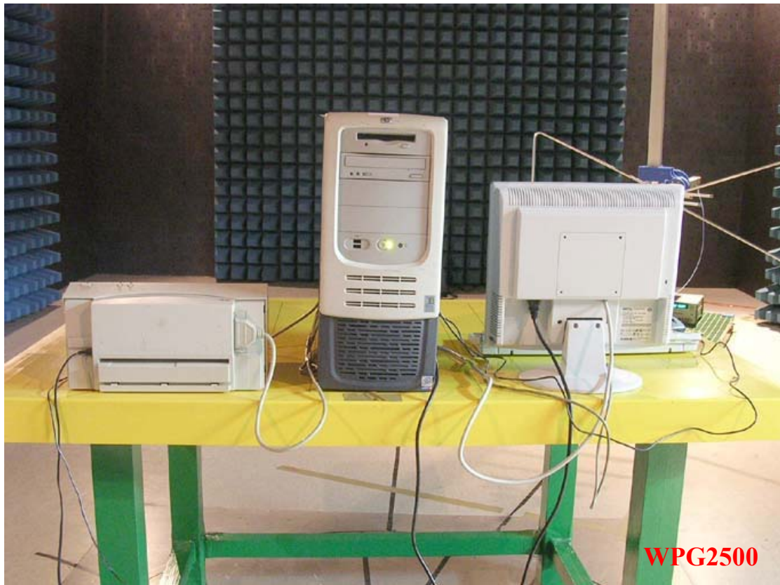
Photo 2: Radiated Emission Test Set-up
