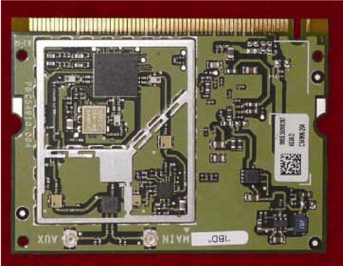
Front with Shielding Removed
