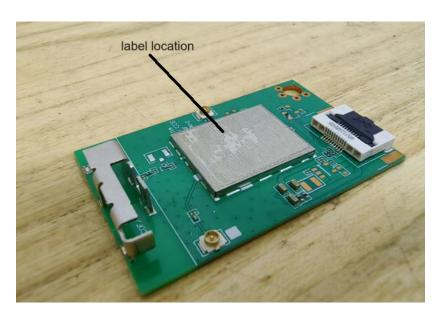
The label is attached to the surface of the shield with a permanent adhesive.
