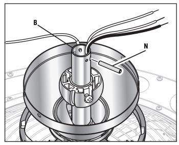
For Canadian installations, refer to the Canada Installation Addendum and install the support cable on the retainer pin (N) now.
