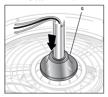
Carefully feed the fan's electrical wiring through the center arm support (E), then install the support (E) with the cupped side facing up.
