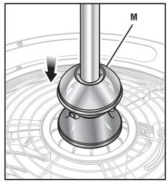
□ Carefully feed the fan's electrical wiring through the canopy screw cover ring (D) and canopy (C), then install the cover ring (D) and canopy (C) on the downrod (B) as shown.
