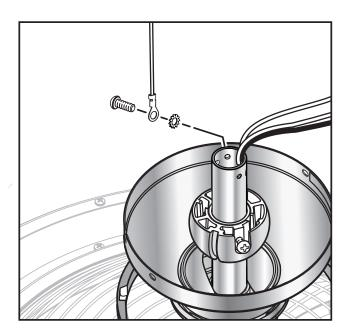
□ Reinstall the retainer pin (N) in the downrod (B).
