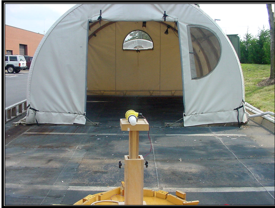
Photograph 11: Radiated Emissions Front View 19.5 dBi Rod Antenna
