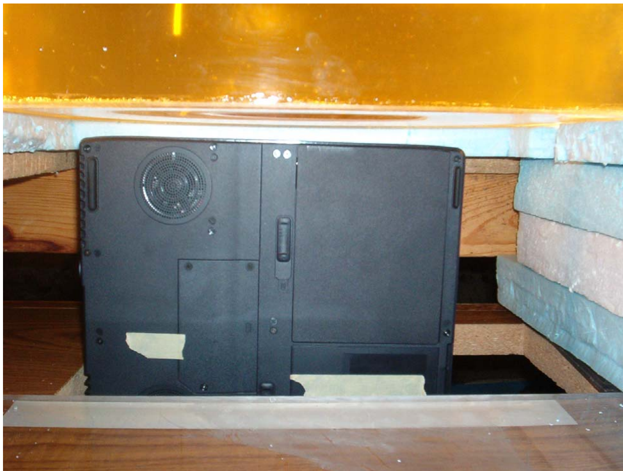
b1. Side view. The left edge with "Aux" antenna at a distance of 1.5 cm from the bottom of the planar phantom.
