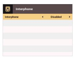
**3** When the intercom is connected, press the ⟨/⟩ buttons to select **Enabled**.
