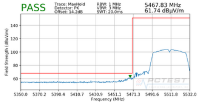
Plot 7-19. Radiated Lower Band Edge Plot (Peak – UNII Band 2C)
