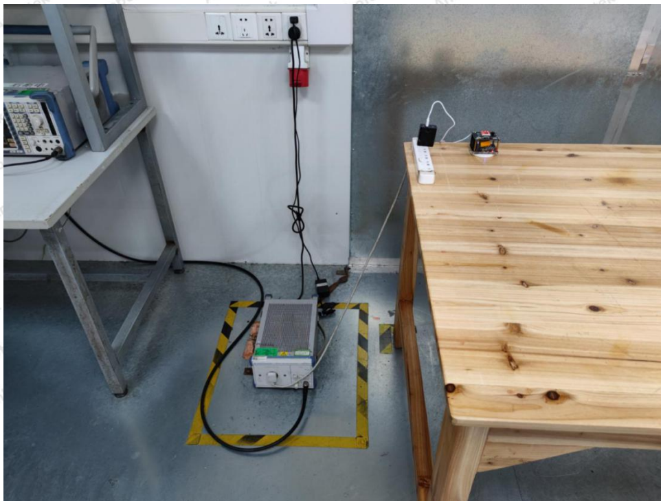
Photo of Conducted Emission Measurement
