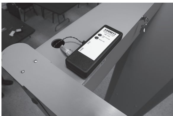
(Above) Wireless Synchronization Module mounted externally.
