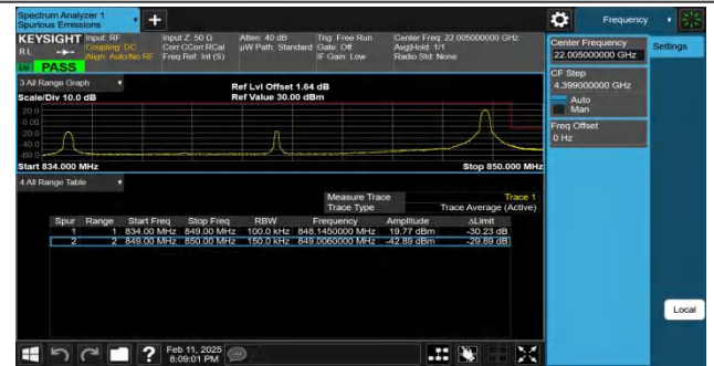
Band26(824-849)-15MHz-QPSK-26965-1RB#74-PASS
