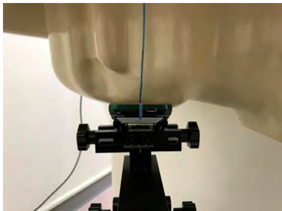
Fig.3 Right Head Section / Cheek-Touch Position
