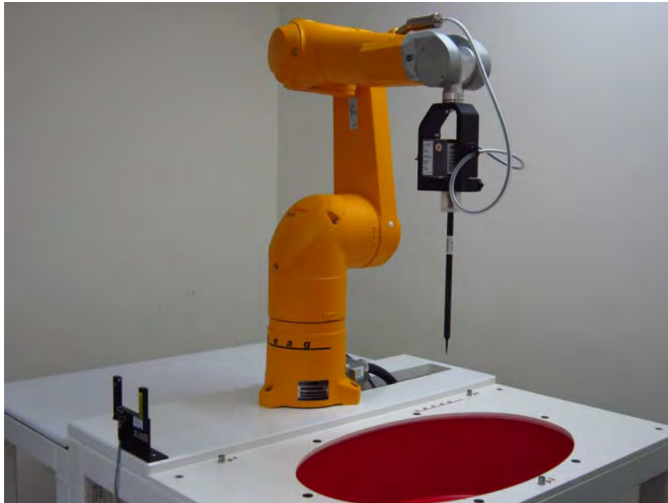
Fig.1 Photograph of the SAR measurement system
