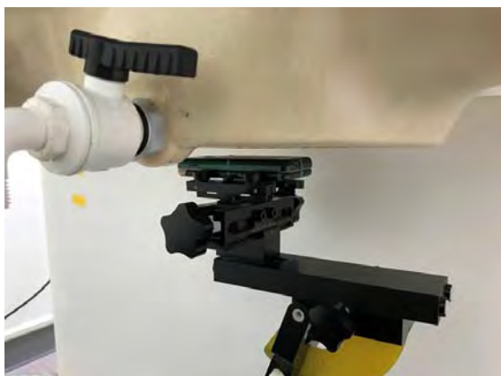
Fig.10 EUT Back side to flat phantom
