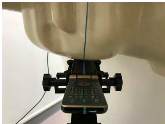
Fig.4 Right Head Section / Ear-Tilt Position(15°)
