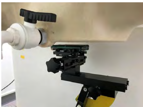
Fig.8 EUT Back side to flat phantom
