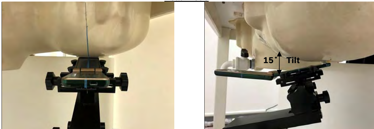
Fig.6 Left Head Section / Ear-Tilt Position(15°)
