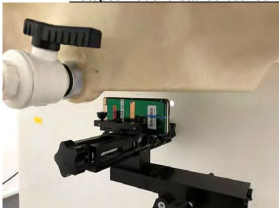
Fig.12 EUT Right side to flat phantom
