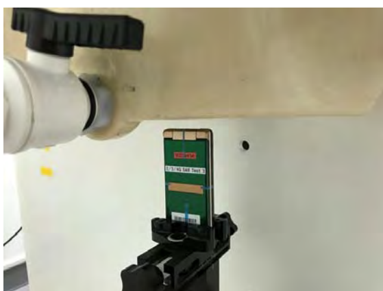
Fig.11 EUT Top side to flat phantom
