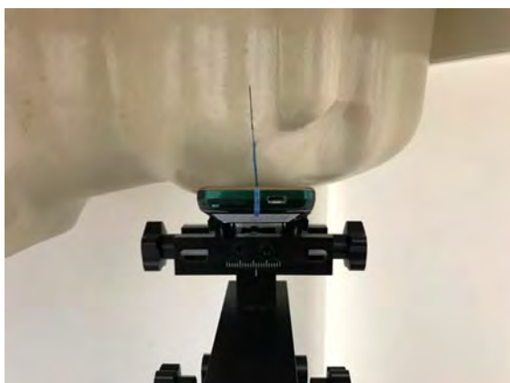
Fig.5 Left Head Section / Cheek-Touch Position
