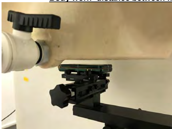
Fig.7 EUT Front side to flat phantom
