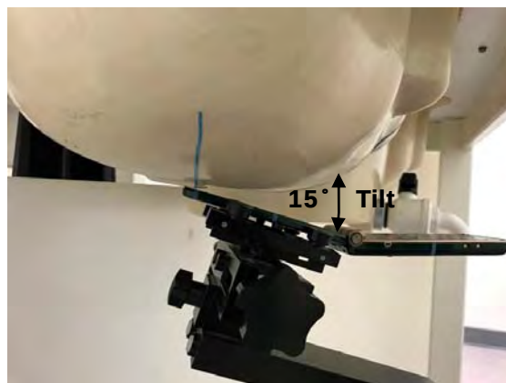
Fig.4 Right Head Section / Ear-Tilt Position(15°)
