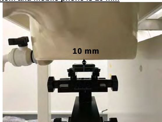
Fig.7 EUT Front side to flat phantom
