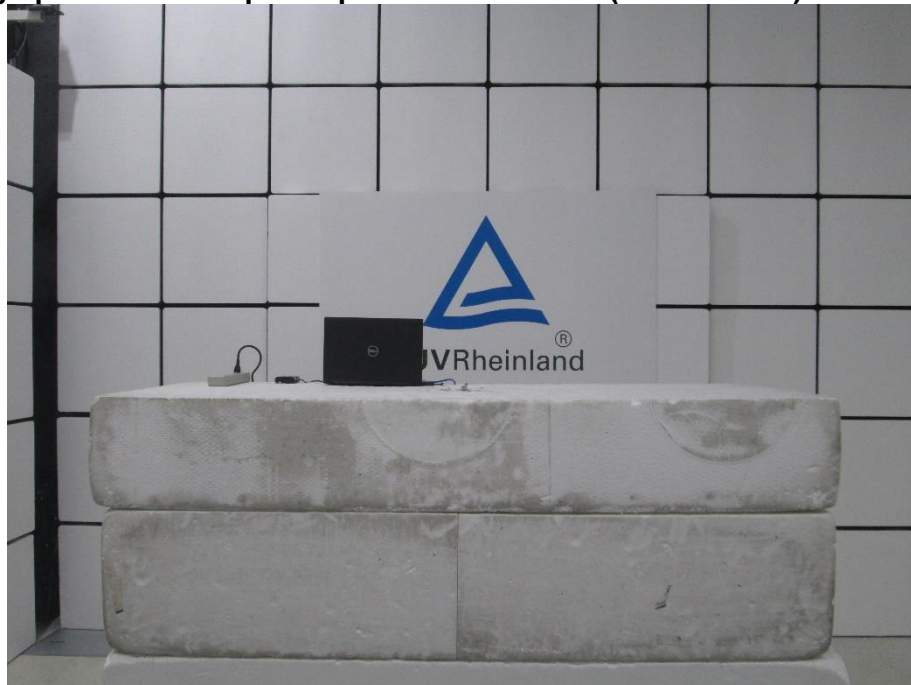
Photograph 2: Test Setup for Spurious Emissions (Front View 2)
