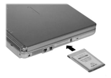
Inserting a PC Card
