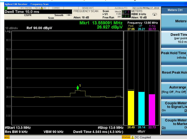
Line 2, 240VAC/50Hz Fundamental Emission with Dummy Load
