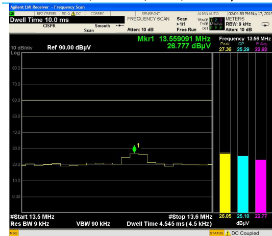
Line 1, 240VAC/50Hz Fundamental Emission with Dummy Load
