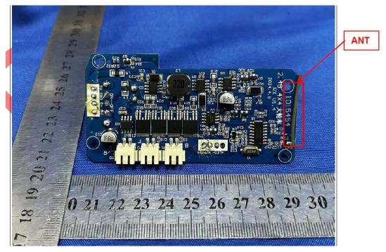
Length: 33mm Antenna Type: Wire Antenna Antenna Gain:-3dBi
