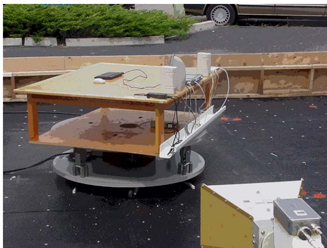
Photograph F.7-2 - Vertical 3115 Horn and LNA Cellular Radiated Emissions Setup
