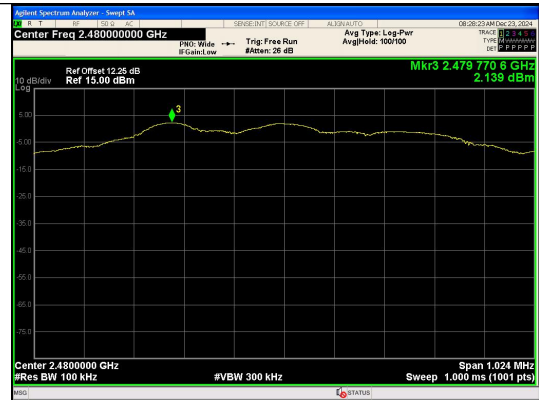
In-Band Reference Level BLE 1M_Channel 39
