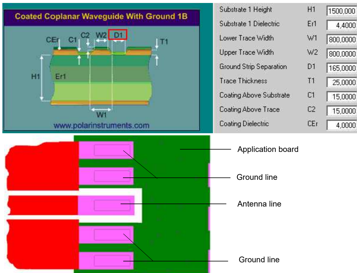
Figure 31: Micro-Stripline on 1.5mm Standard FR4 PCB - example 1
