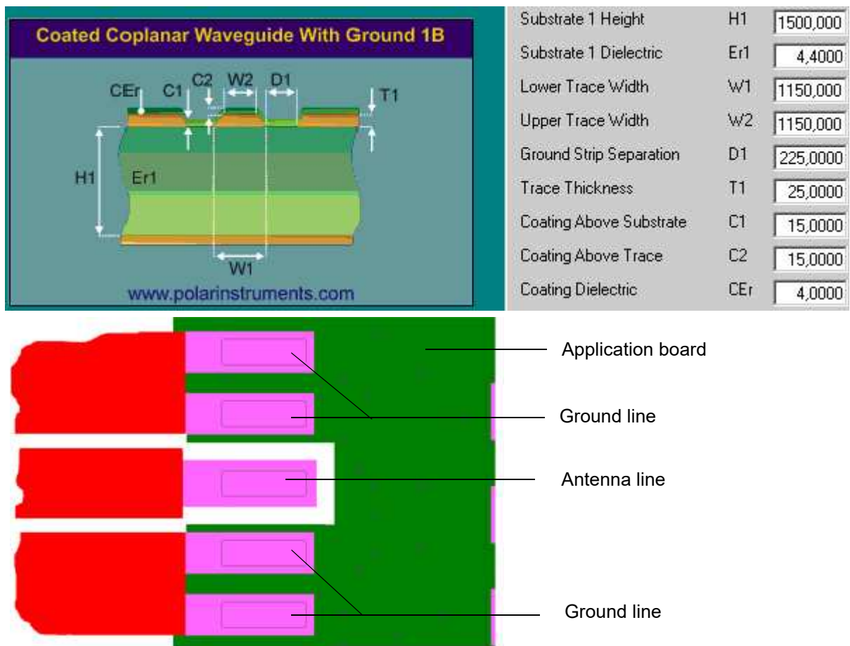
Figure 32: Micro-Stripline on 1.5mm Standard FR4 PCB - example 2
