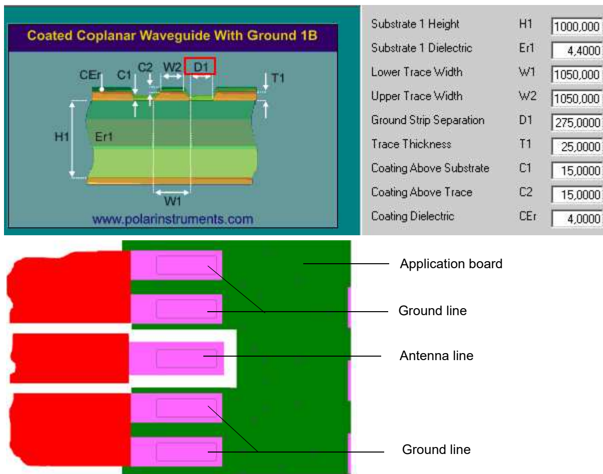
Figure 30: Micro-Stripline on 1.0mm Standard FR4 PCB - example 2
