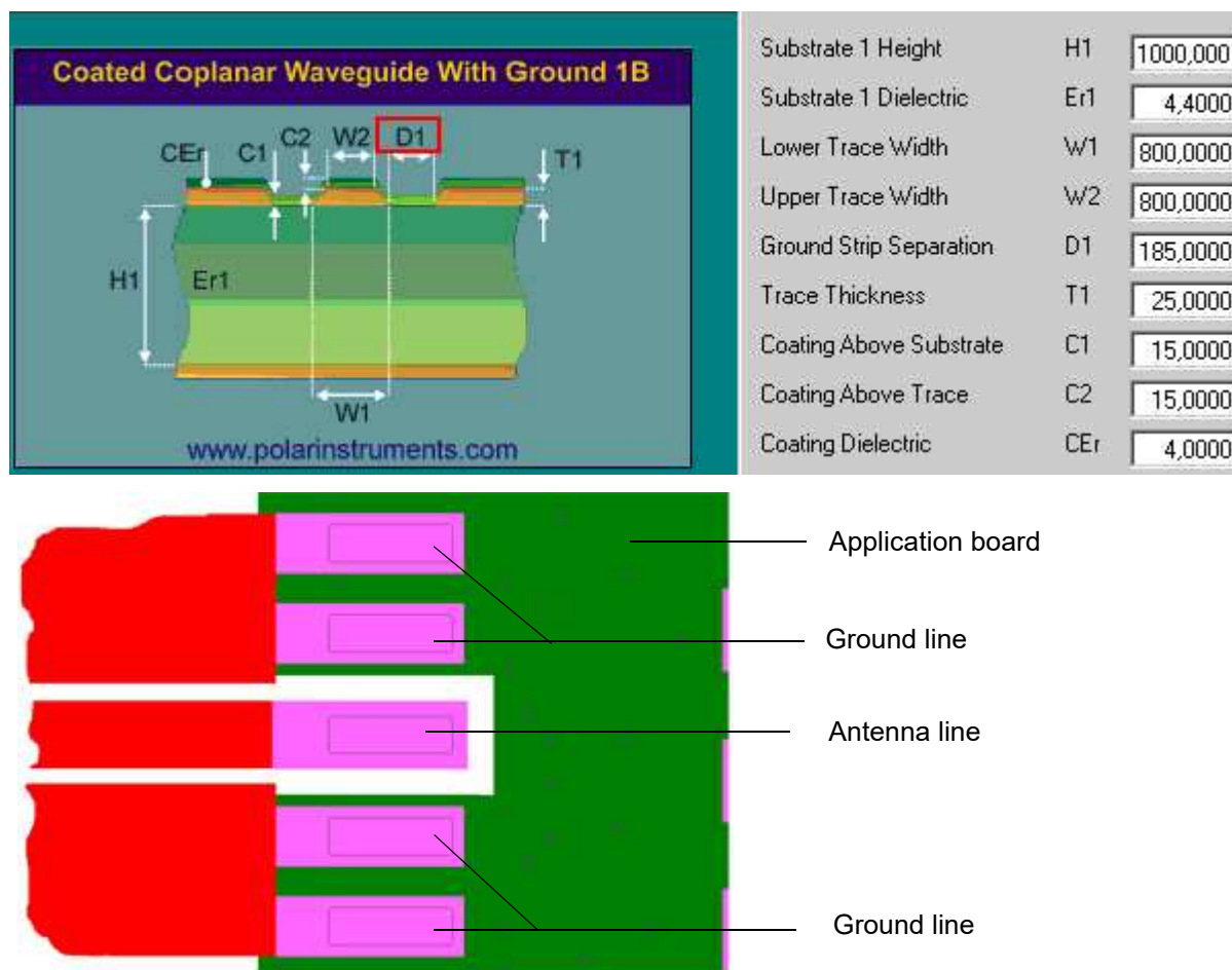
Figure 29: Micro-Stripline on 1.0mm standard FR4 2-layer PCB - example 1
