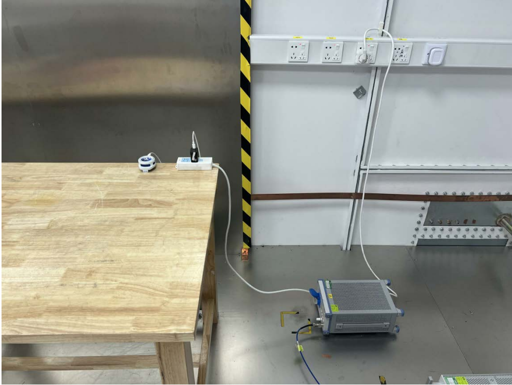
AC Power Line Conducted Emission
