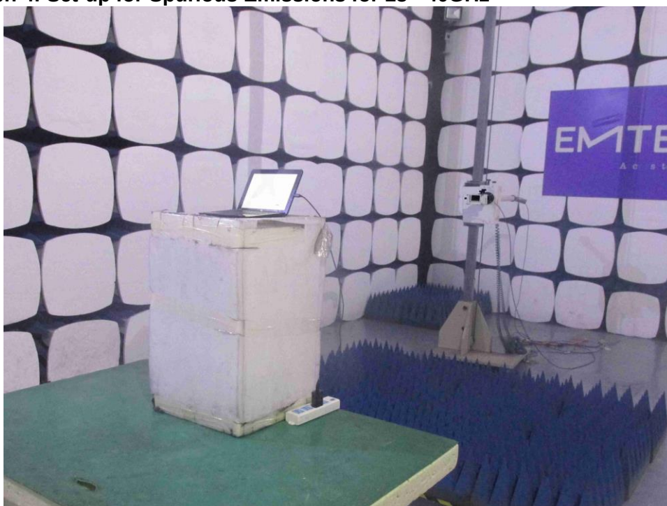
Photograph 4: Set-up for Spurious Emissions for 18 - 40GHz
