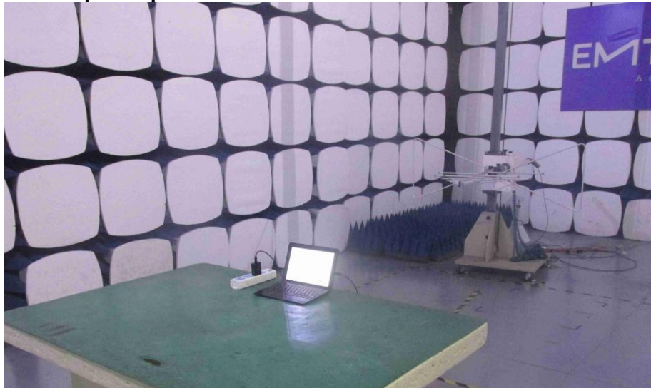
Photograph 2: Set-up for Spurious Emissions for 30 - 1000MHz
