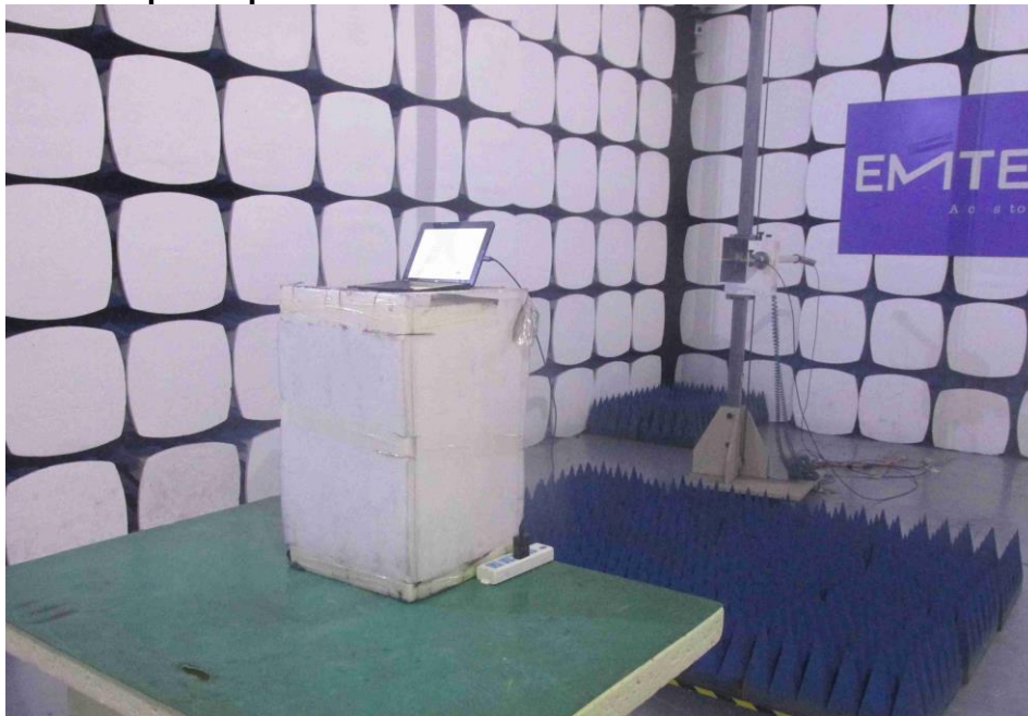
Photograph 4: Set-up for Spurious Emissions for 18 - 40GHz
