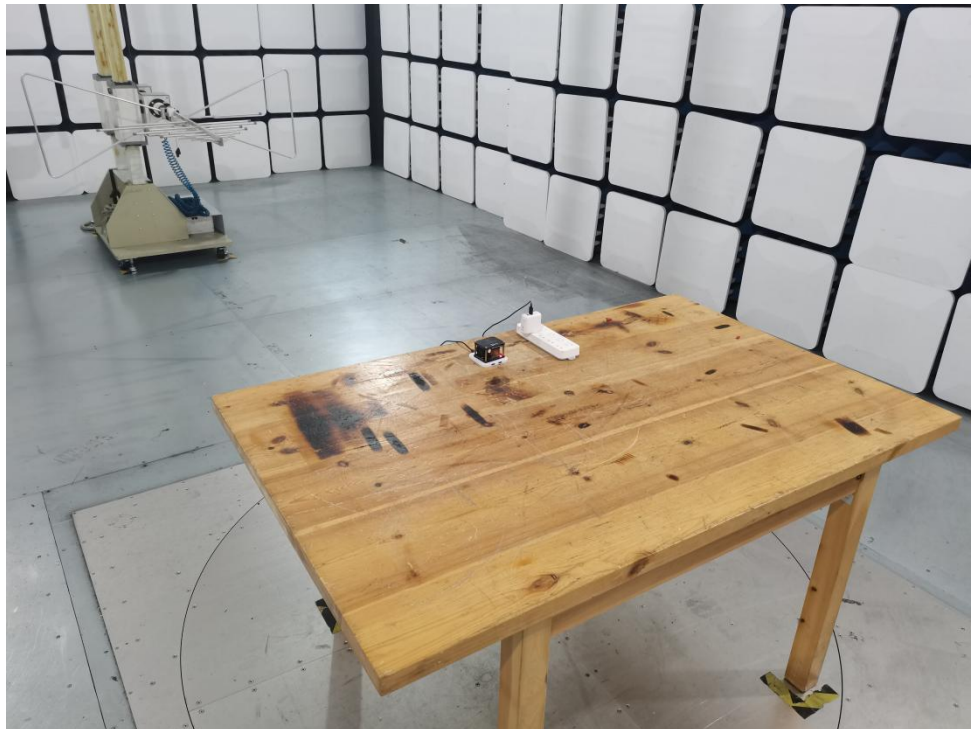
Photo of Radiation Emission Test
