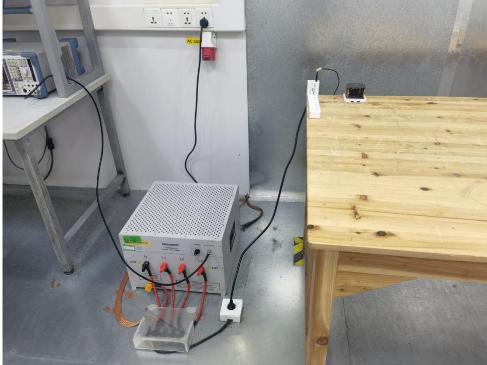
Photo of Conducted Emission Measurement
