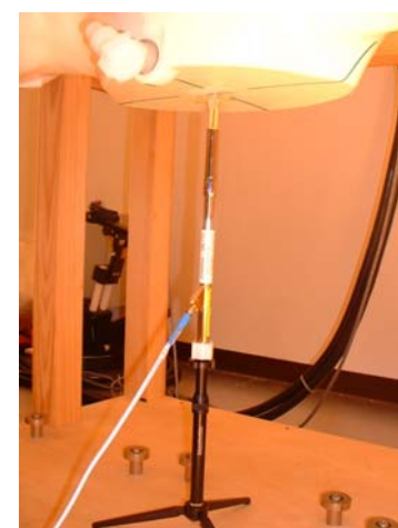
2450MHz System performance check setup
