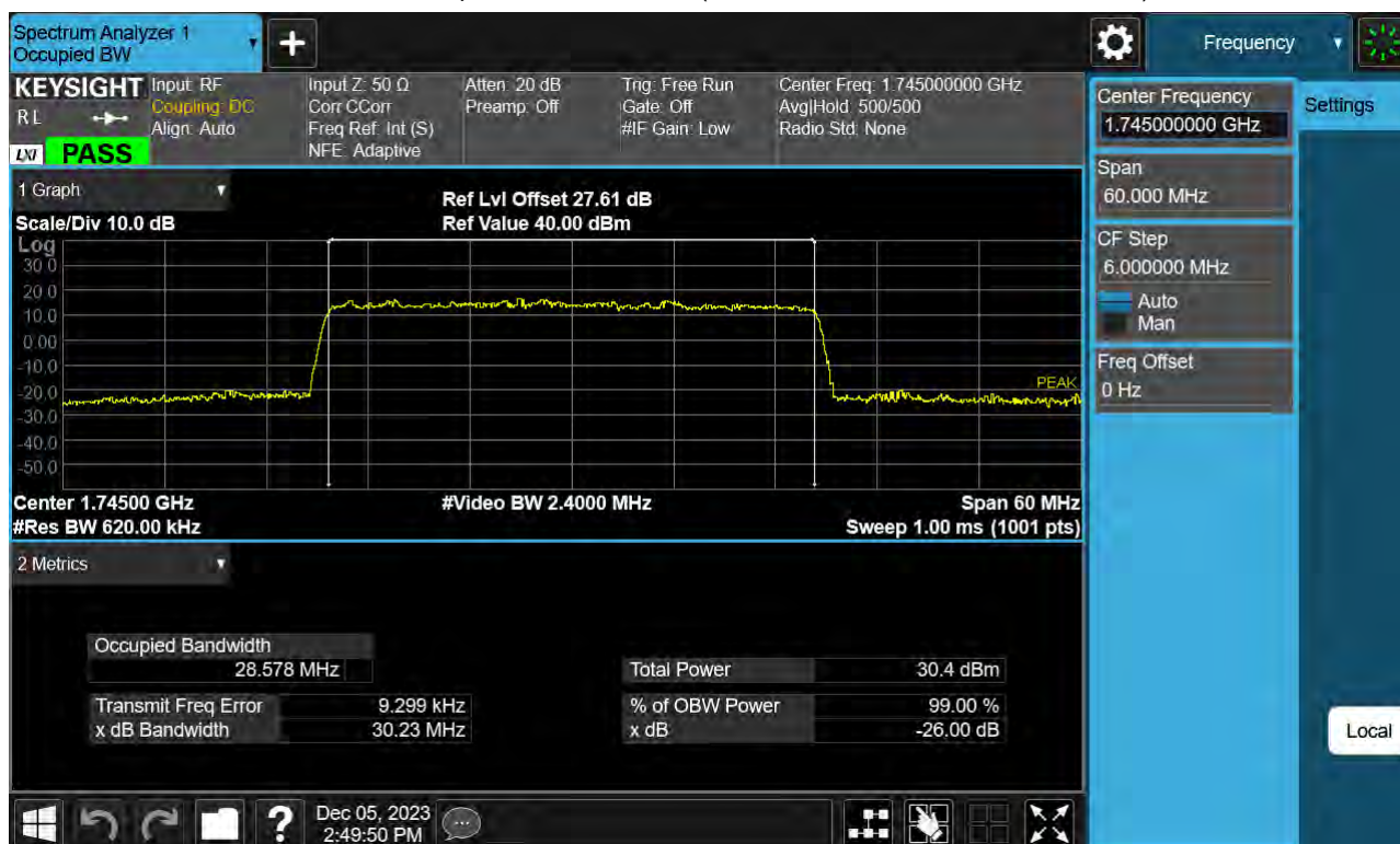
Sub6 n66. Occupied Bandwidth Plot (30 M BW Ch.349000 64QAM Full RB)
