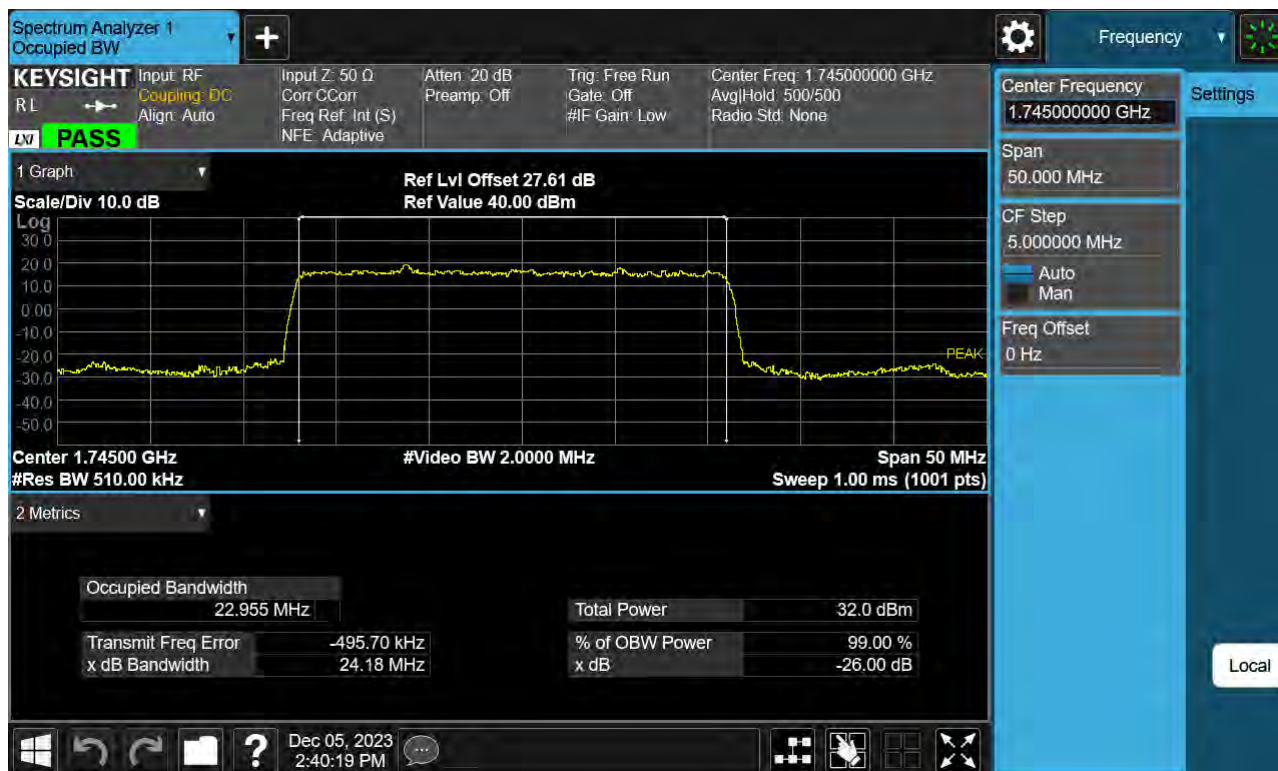
Sub6 n66. Occupied Bandwidth Plot (25 M BW Ch.349000 BPSK Full RB)
