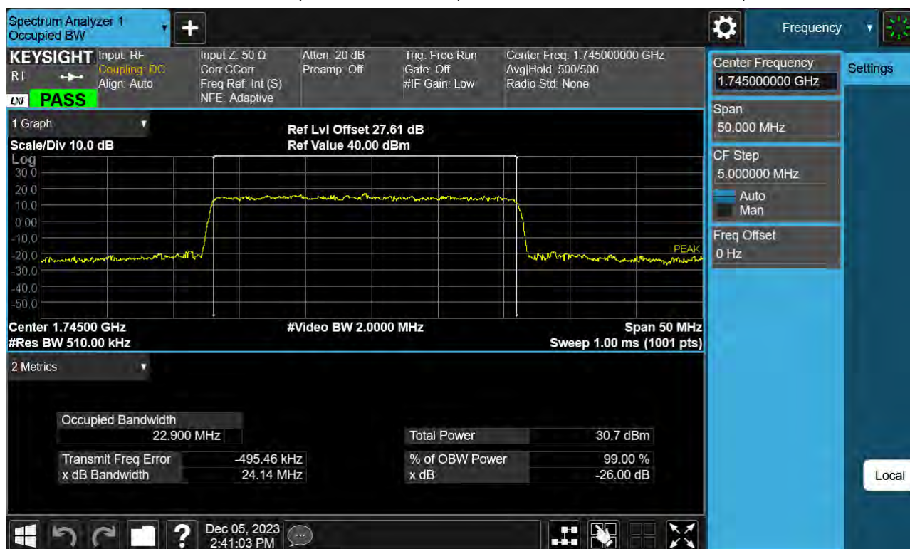
Sub6 n66. Occupied Bandwidth Plot (25 M BW Ch.349000 16QAM Full RB)
