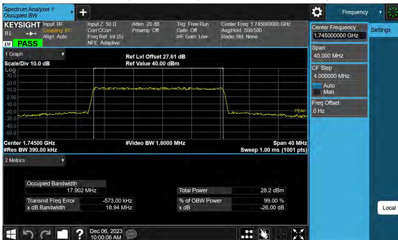
Sub6 n66. Occupied Bandwidth Plot (20 M BW Ch.349000 256QAM Full RB)
