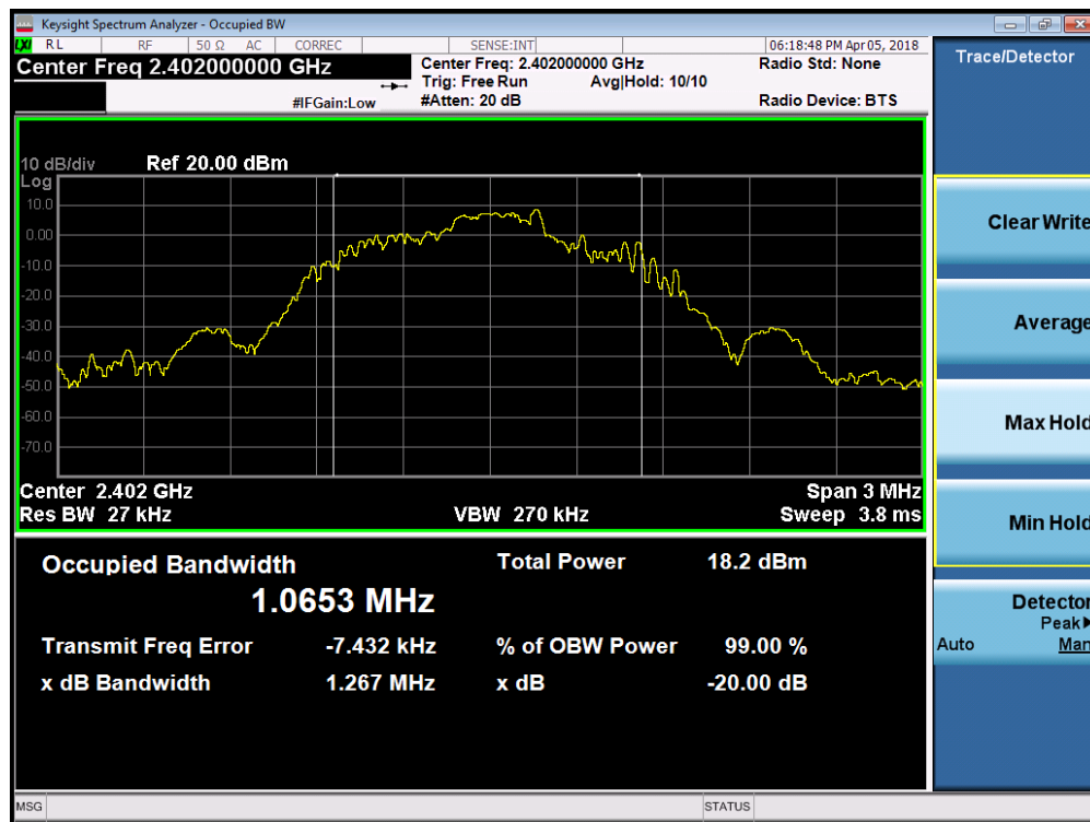
Plot 7-1. 20dB Bandwidth Plot (Bluetooth, 1Mbps – Ch. 0)
