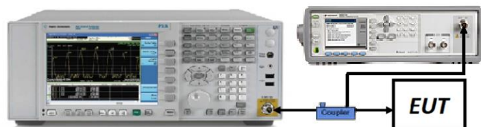
Figure 7-3. Test Instrument & Measurement Setup
