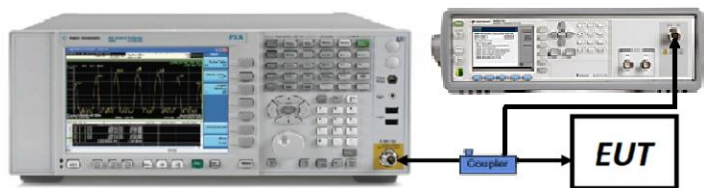
Figure 7-4. Test Instrument & Measurement Setup
