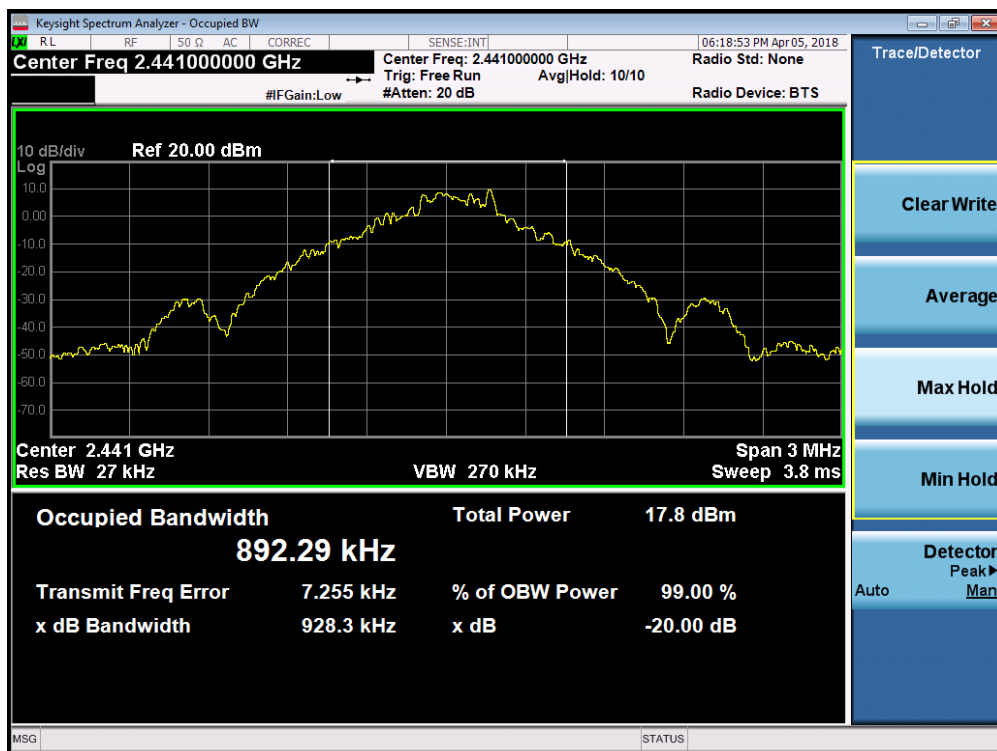
Plot 7-2. 20dB Bandwidth Plot (Bluetooth, 1Mbps – Ch. 39)
