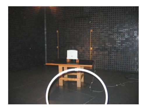
Photograph No.3 Radiated emissions measurement setup in the anechoic chamber in 30 -1000 MHz
